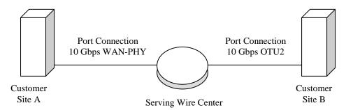
This example illustrates a same speed/different format circuit configuration whereby there is a 10 Gbps WAN-PHY Port Connection between Customer Site A and the serving wire center and a 10 Gbps OTU2 Port Connection between Customer Site B and the serving wire center. In this circuit example, both a 10 Gbps WAN-PHY and a 10 Gbps OTU2 Port Connection charge would apply.
