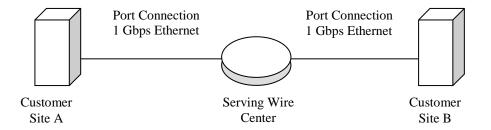
This example illustrates a 1 Gbps Ethernet circuit from Customer Site A to Customer Site B for a same speed/same format arrangement. In this example, two -1 Gbps Ethernet Port Connection charges are applicable.
