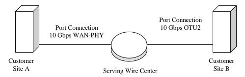
This example illustrates a same speed/different format circuit configuration where there is a 10 Gbps WAN-PHY Port Connection between Customer Site A and the serving wire center and a 10 Gbps OTU2 Port Connection between Customer Site B and the serving wire center. In this circuit example, both a 10 Gbps WAN-PHY and a 10 Gbps OTU2 Port Connection charge would apply.
